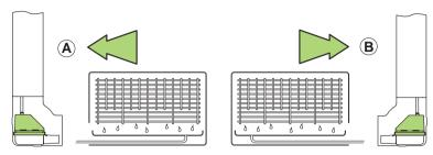
Disassemble system. Hold 'Elbow back', 'Internal conduit sleeve' and 'Conduit back' against the wall, squaring up to th ceiling and the evaporator unit. Drill fixing holes in wall and secure using rawl plugs and screws supplied.
