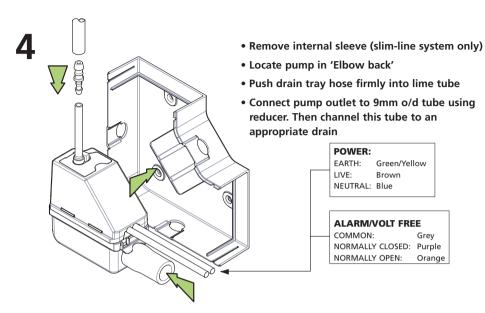
Wire the Mini Lime Pump to the permanent Live, Neutral and Earth terminals of the Evaporator. Install a 1.0 amp in-line fuse between the Mini Lime Pump and the Evaporator.
