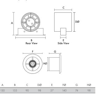
Internal/External Grille Dimensions 140x140mm Fan Transformer (W x H x D)  $87 \times 87 \times 33$
