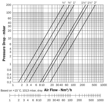
Based on f = 1.24 Natural Gas Flow - Nm<sup>3</sup>/h
