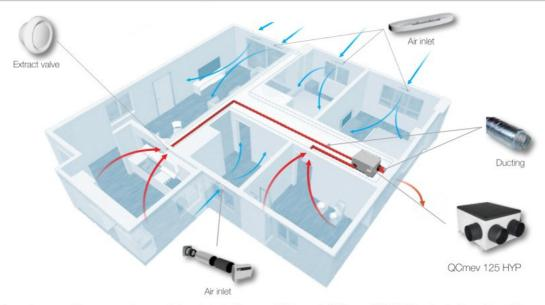
How it works: a continuous running centralised single flow ventilation unit (QCmev 125 HYP) extracts the stale air from different rooms contemporaneously, with top acoustic comfort.
