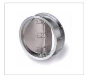
Automatic duct shutter **RVS 250** Ref. no. 02592 With spring return, can be installed horizontally in any direction, vertically with throughflow from bottom to top. Shutter opening in flow direction; automatic function through fan operation.
