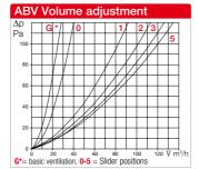
The throughflow depending on the setting and underpressure is shown in the diagram above.
