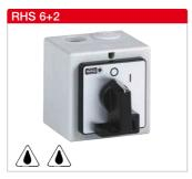
RHS 6+2 Ref. no. 01595 "0" position can be locked with a padlock. In accordance with DIN EN 60204 p.1/VDE 0113-1. Plastic casing for surface-mounted installation. 6-pole with 2 auxiliary contacts, for all pole-changing fans.
