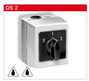
DS 2 Ref. no. 01351 Speed switch and on/off switch for two-speed three-phase current fans in Y/△ connection. Grey plastic casing for surface-mounting.
