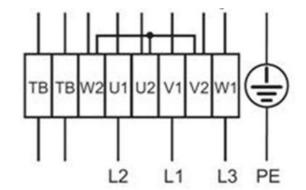
High speed Low Speed  $\Delta$ -Connection Y-Connection
